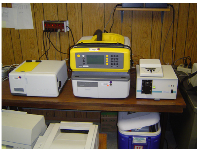
Fig. 1. Photograph presenting a typical instrument layout in a field laboratory. The pictured HAPSITE GC-MS sits at the centre and is equipped with conventional headspace (left) and MAP-HS apparatus (right). The current MAP-HS configuration is not specific to HAPSITE and it is operated via a remote controller (that is located on top of the MAP-HS in this picture).
